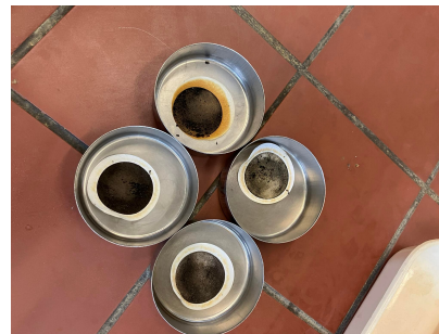
(b) OM remaining after the second attempt to remove OM using Fenton's reagent.
